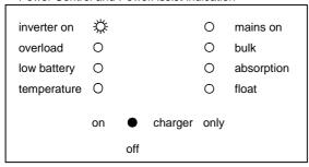
**Note:** When the LED's "overload" and "low battery" are on simultaneously, the Multi(Plus) or Inverter Compact has switched off due to excessive DC ripple voltage.
