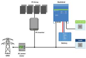
**Grid parallel topology with PV inverter** Similar to Hub 4-2 but in this topology the PV inverter will shut down in case of
